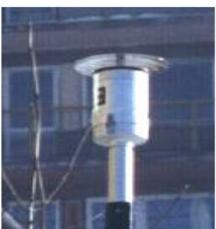
In place of standard air inlet a PM-10 or PM-2.5 air inlet can be installed cutting off dust with particle size greater than 10  $\mu\text{m}$  (PM-10), greater than 2.5  $\mu\text{m}$  (PM-2.5) See the picture at left. The air inlets PM-10 and PM-2.5 are optional.
