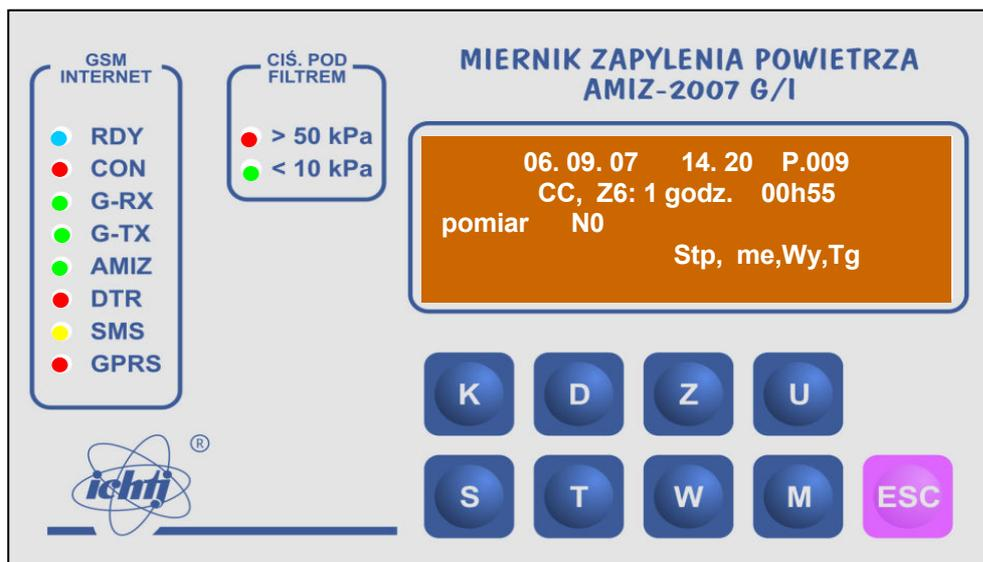
Fig. 4. Keyboard, display and LED control indicators
