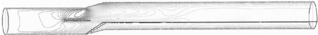
Fig.2. Contours of velocity magnitude for guide vanes parallel to the reactor axis.
