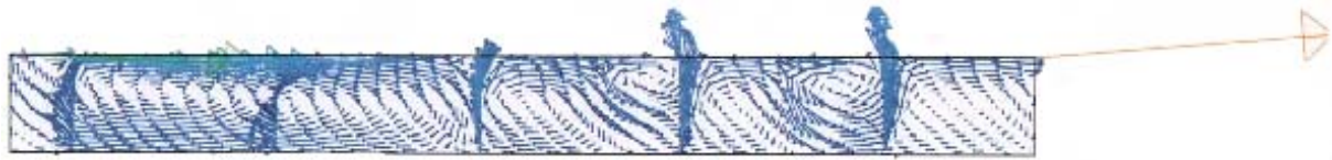
Fig.2. Flow structure and velocity field for water flow rate Q_w = 2.7 \text{ m}^3/\text{h} , Q_a = 3 \text{ m}^3/\text{h} .
