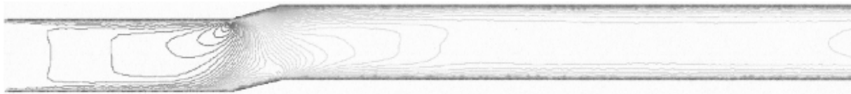
Fig.1. Contours of velocity magnitude for lifted bottom of reaction chamber.
