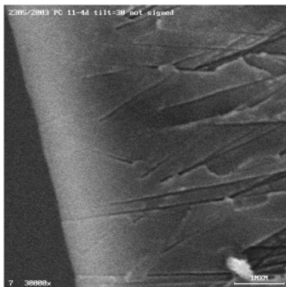
Fig.2. Fracture through the PC particle track membrane.
